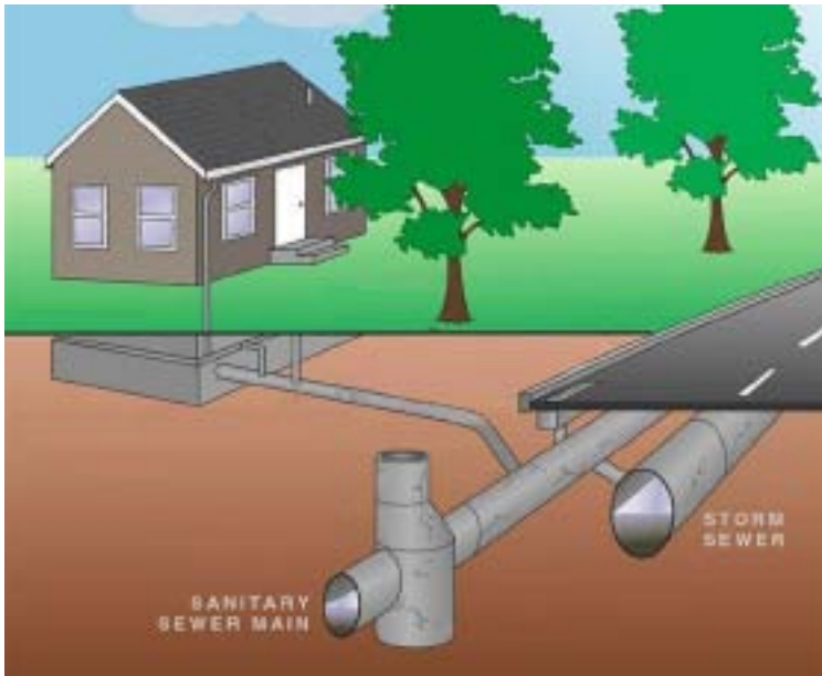
FIGURE 3 - SANITARY SEWER SYSTEM
